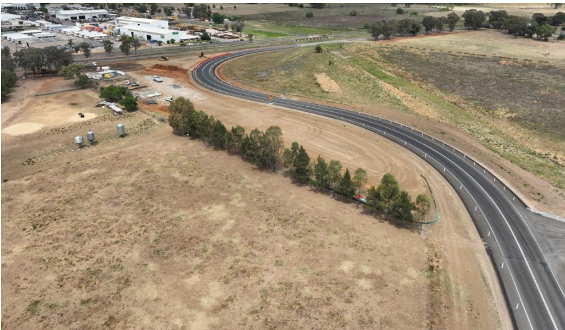
Figure 2 – Tie-in of the Jewry Street extension with Wallamore Road to the west of the new roundabout (view is to the southwest).
